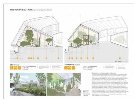
Image 7: Design in section: dry and temperate biomes.
