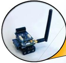
The Wireless Sensor used in this project. It is equipped with a three axial accelerometer able to measure up to 256 samples per second. Assuming that it performs a measurement 6 times a day, it consumes only 440  $\mu$ J per day.
