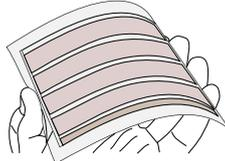
The cell is combined with a proper electronic and energy storage circuit which helps realize the development of a sensor prototype. Another attractive advantage of thin-film solar cells is their flexibility as the cells can be shaped in various ways or simply glued to the structure.
