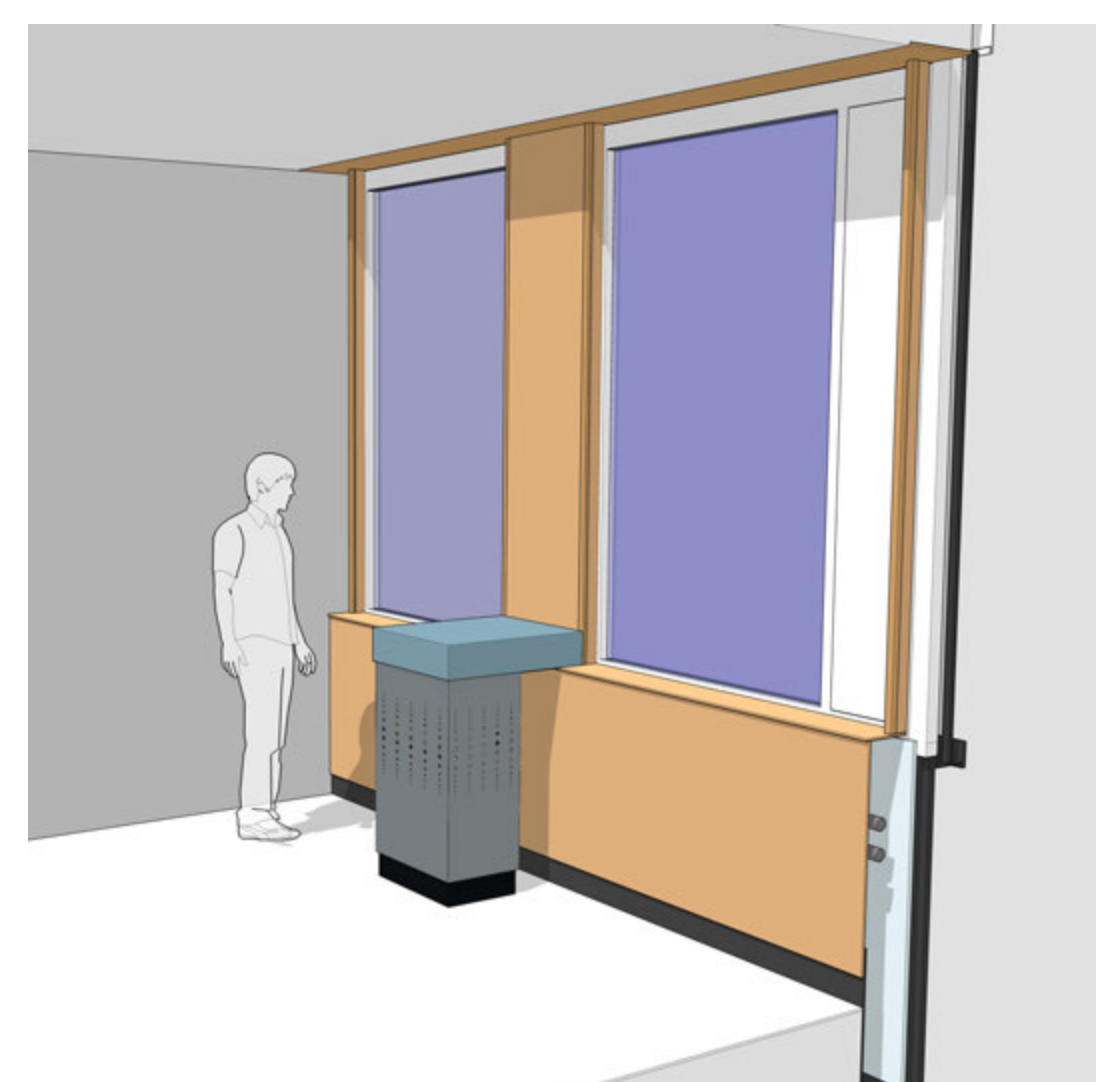
Interior of facade with new casing and decentralized air intake
