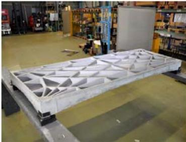
Innovation matters - building lightweight unreinforced concrete slabs by learning from the Guastavino vaults eliminates 70% of the material and energy while enabling passage for thermal conditioning or networking.
