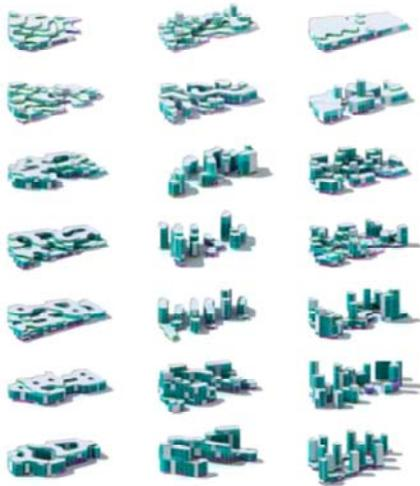
Figure 2: While using the same space allocation plan, different architectural layouts are generated, dependent on the weighting of the various qualities (e.g., view, length of paths, insulation, provision of vertical accessibility); the layouts are shown as 3-D-models here.
