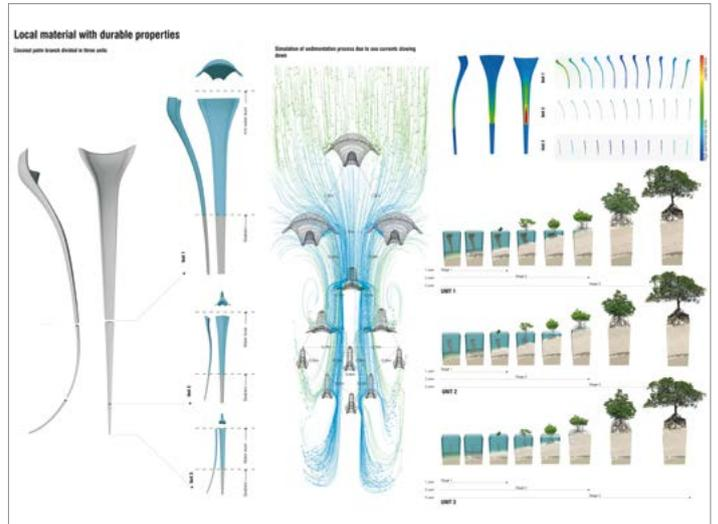
Image 2: Material system: structure and performance. Palm branches have an ideal “spoon” shape which enables a sea current to slow down and deposit sand material in the concave area of the unit. In this way mounds of sand deposit are created, which gradually create a higher coastline. During the process, the palm branch transforms to “geoarmature”, which is able to host aquatic plants, like mangroves.
