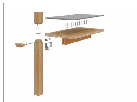
Image 9: Framework, exposed two-hour-rated connection.
