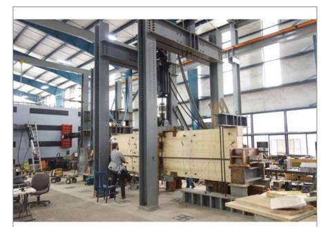
Image 10: Framework, CLT rocking wall testing.
