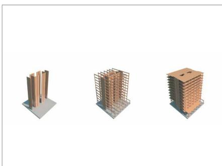
Image 7: Framework, timber core, framing, and floor.
