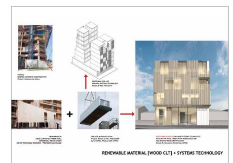
Image 10: Innovation - EcoSyst - Adaptable prefabricated cluster components using machined mass timber panels.
