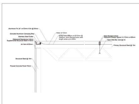
Image 3: Prototype structure: A simple construction supports 10mm water layer atop 97 % transparent ETFE foil.
