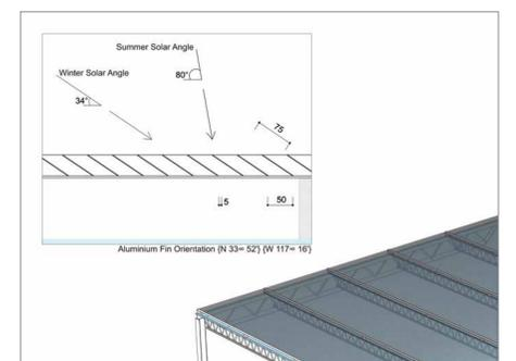
Image 6: Aluminum fin orientation: Shades water for max. cooling during summer but max. daylighting in winter.
