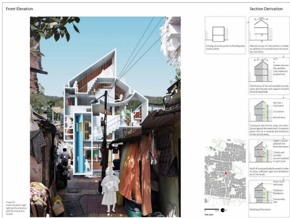
Image 2: Left: Front elevation (design proposes a new playful elevation that follows differing proportions to respond to the varying anthropometric needs of its users). Right: Section evolution diagram and site plan.
